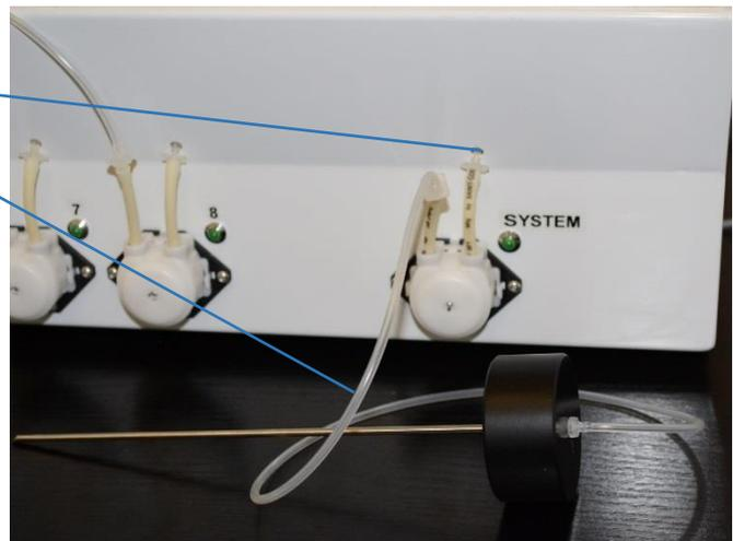
Connection between the pump and the bottle cap of the system solution (21) including the pump tube connector.
