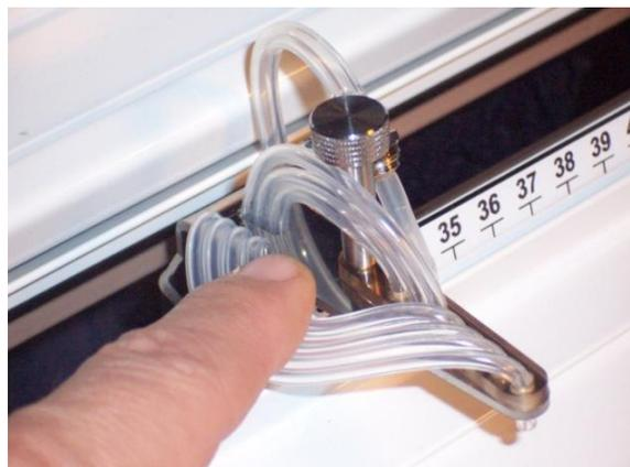
The tubes C,D,G are inserted in front of the arm pivot, A,B,E,F behind it.
