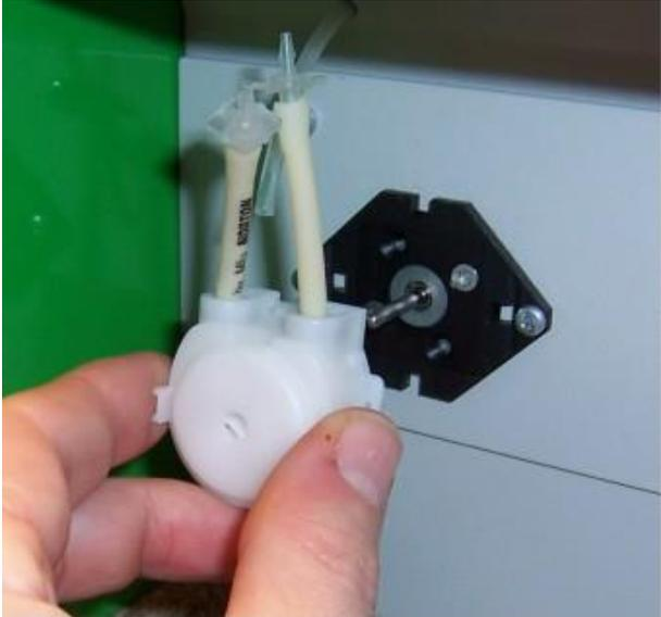
Equip the new head tube by 2 pieces tube-to-tube connector (AC-6). Push the black tool to hole in the front side of the head and mount the head on the motor shaft. Také care to get back the lock well.
