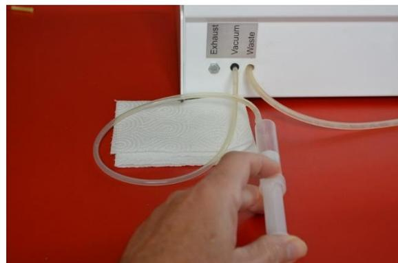
5. Empty the beaker (to prevent its overflow) and repeat the step 4 with distilled water.
