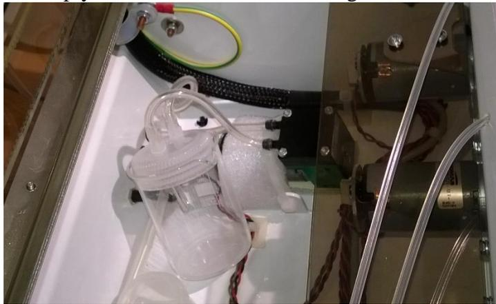
2. Remove the Vacuum tube from the waste bottle.
